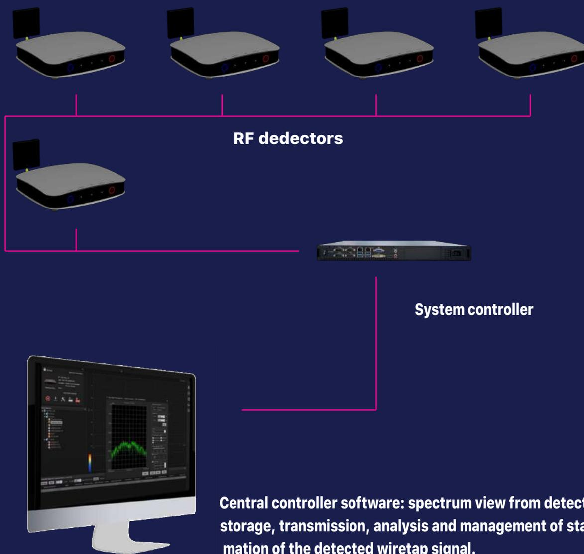
Central controller software: spectrum view from detection terminals, storage, transmission, analysis and management of statistical information of the detected wiretap signal.
