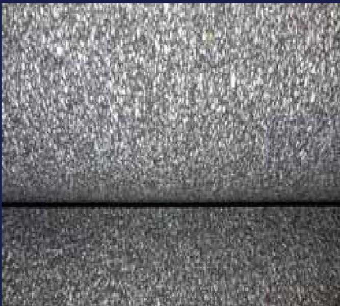
Flexible mat, pressed and compacted, made of polyurethane foams type T3037SG, designed for sound absorption and acoustic insulation.
